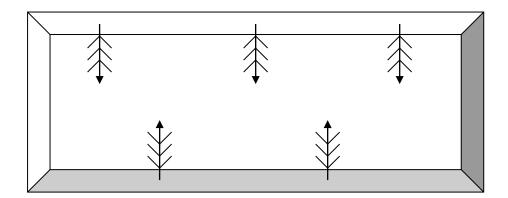
Base area 20 r.m. length x 5 r.m. width =  $100 \text{ m}^2$  (Conductive points should not diverge more than 5 m from each other)
